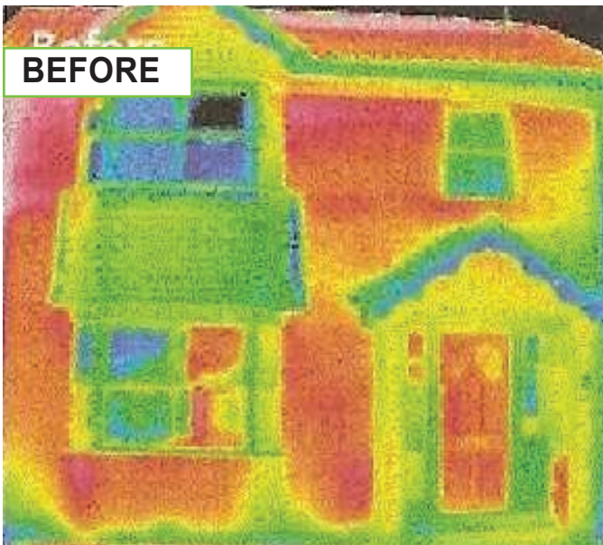
Untreated substrate, high levels of heat loss (Red)
